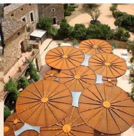
Shelter to have flat, round roof structure with a series of minimal structural posts near the edge. Intention to be non-imposing, non-directional and appear to be a flattened umbrella / parasol as a design cue for the 'weather' in Weatherston.
